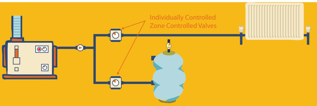
Dividing the heating system into separate zones allows it to operate independently in different parts of your house. Typical zones might be (i) the living room, (ii) the rest of the ground floor, (iii) the first floor, and (iv) the domestic hot water storage cylinder. Each zone will be switched on only at the times when there is a demand for heat in that area.
